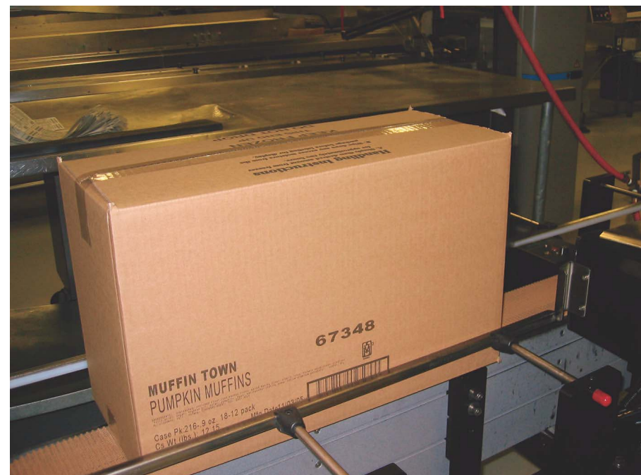
The cases are coded with at least eight lines of text per side that includes product and manufacturing data and an I 2 of 5 bar code.
