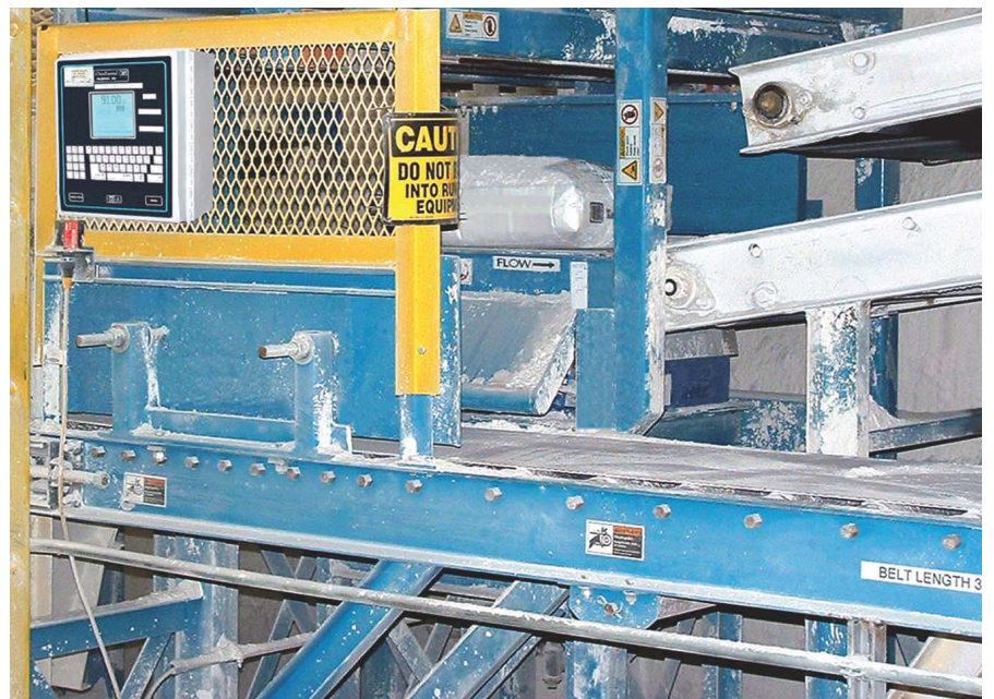
The new-heavy duty checkweigher is specifically designed for the harsh, abusive, dirty environments found in the cement, soil, bark and carbon-black products industries.
