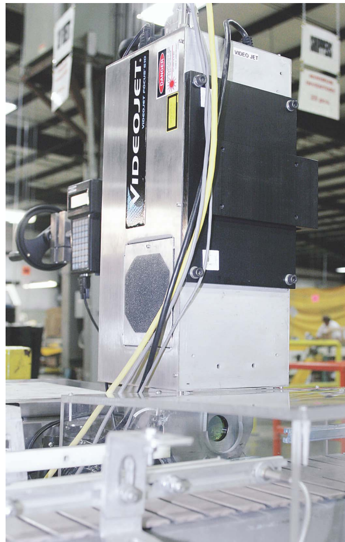
Laser coding packages using the system above complements CCB's available printing services and provides a crisp, clear imprint.
