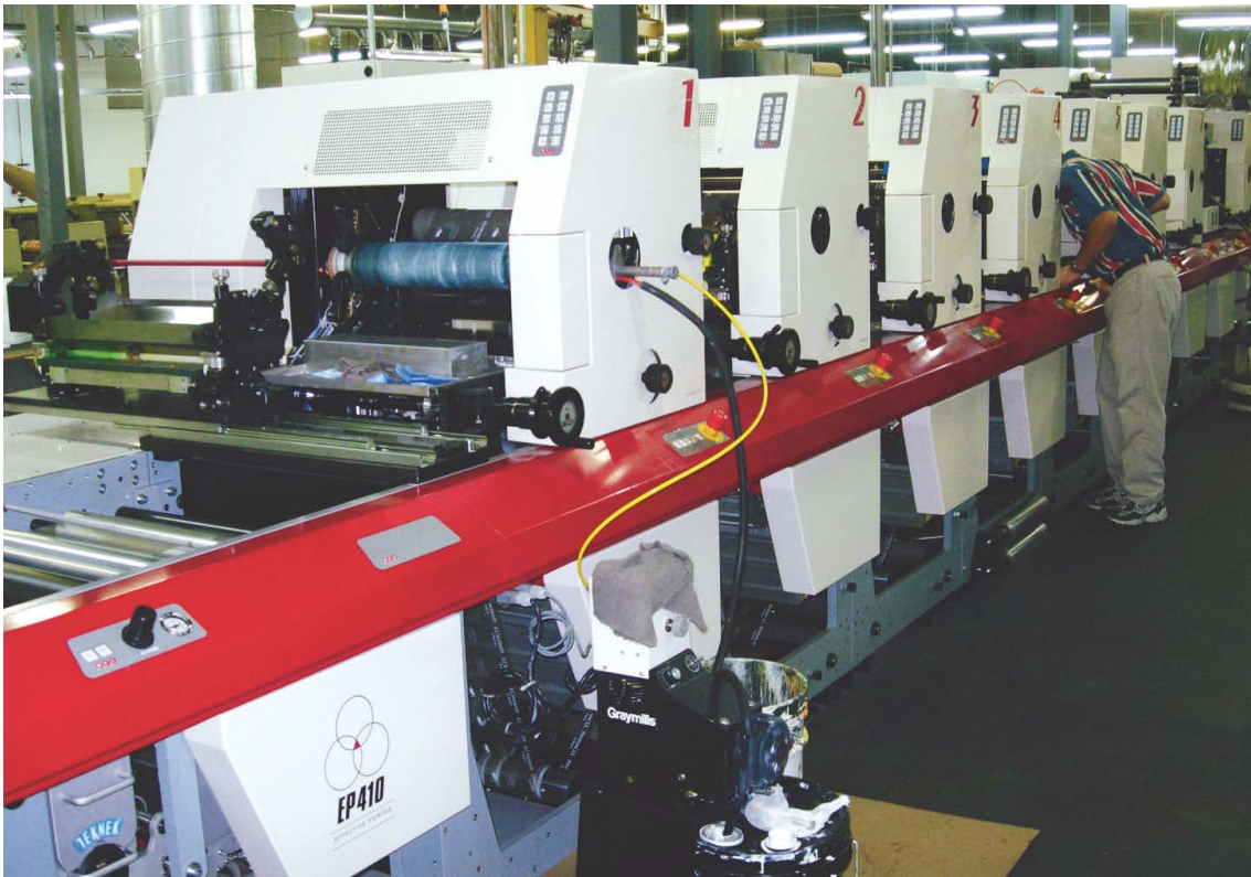
To support its label business, last spring J.R. Cole added a new 16-in., eight-color flexo press, above, at the Labeltec facility. Its latest equipment is a 16-in. inspection slit/rewinder, right, stationed at its Pharmaprint plant.
