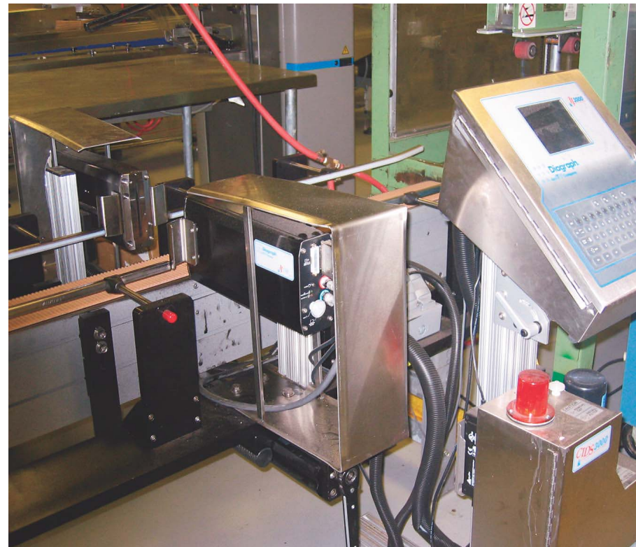
The ink-jet printer, a companion graphical user interface and a color touchscreen are in place on Muffin Town's main packaging line, above. A second unit will be added this year.
