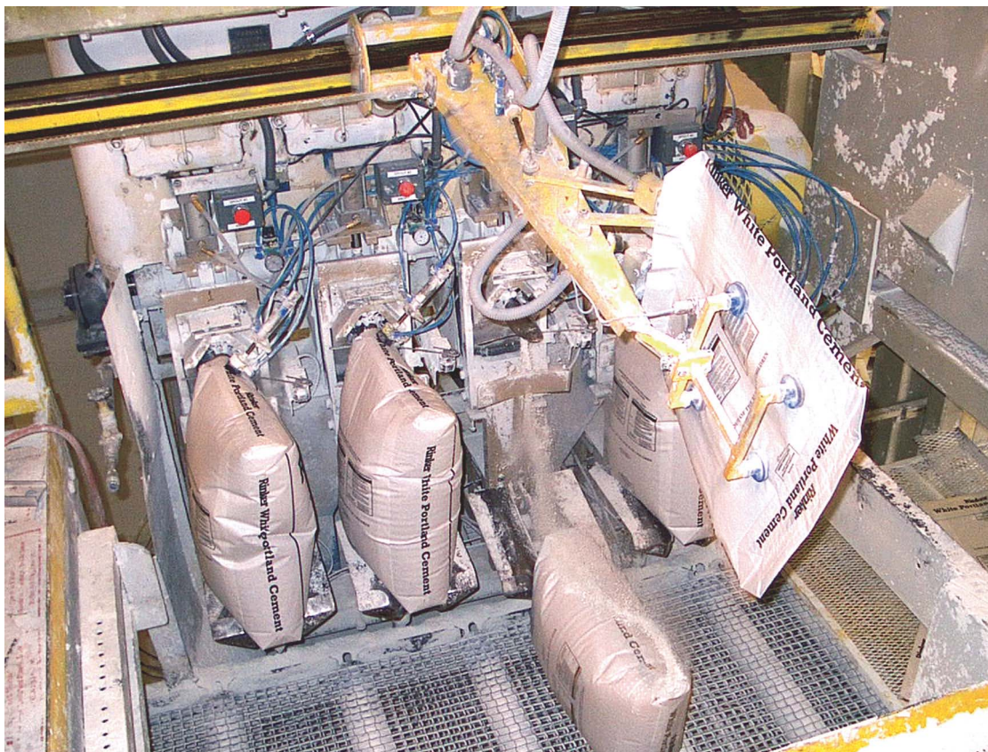
The bag filler was upgraded to a system with automatic controls and a loadcell for more efficient use of older technology. Filling time has improved from 12 to 15 sec/bag previously to 8 or 9 sec/bag now.
